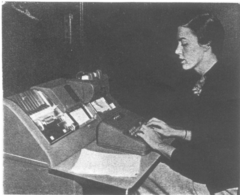
Sentences in Russian are punched into standard cards for feeding into the electronic data processing machine for translation into English
